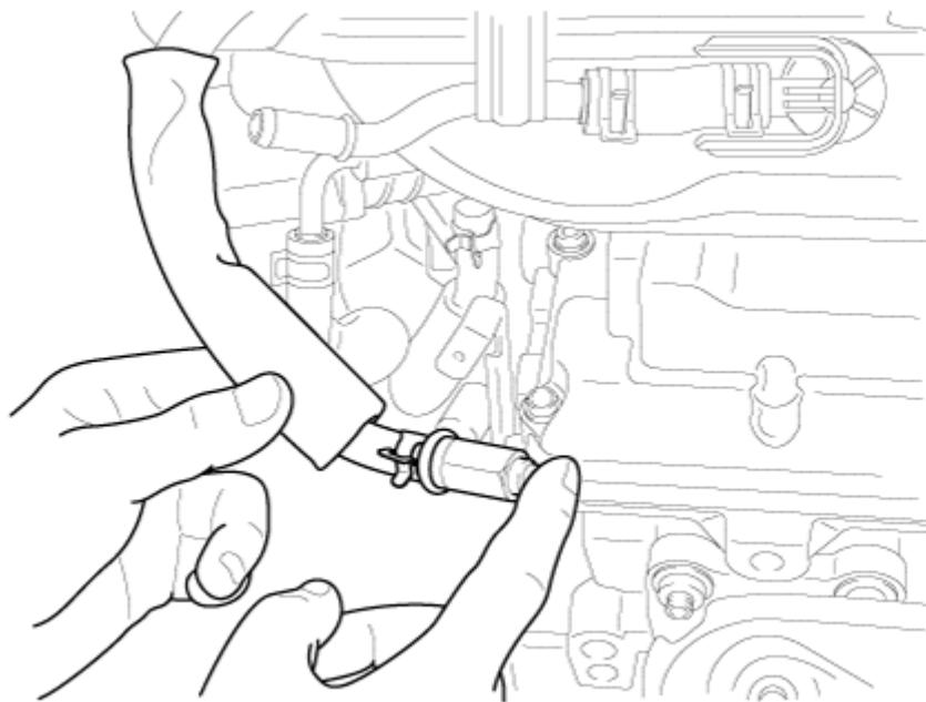
4. If vacuum is not felt, inspect PCV operation. If operating correctly, clean or replace the vapor hose.
